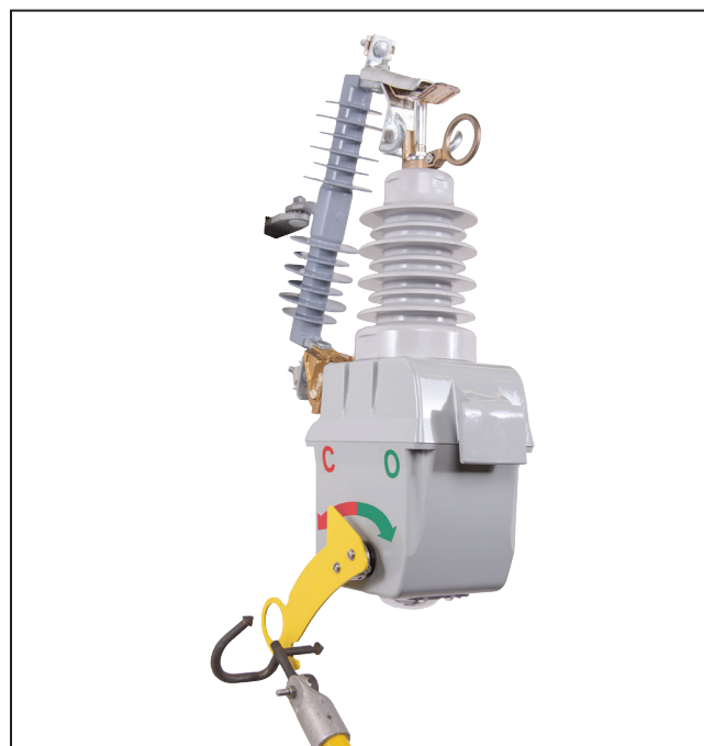
Figure 15. Opening the VacuFuse interrupter by pushing up on the OPEN/CLOSE lever.
