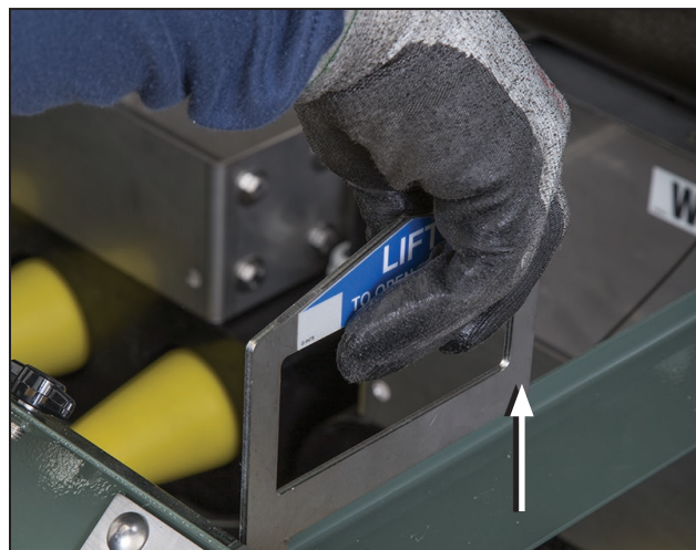
Figure 14. To gain access to the termination compartment, lift the latch handle to open the right-hand door.
