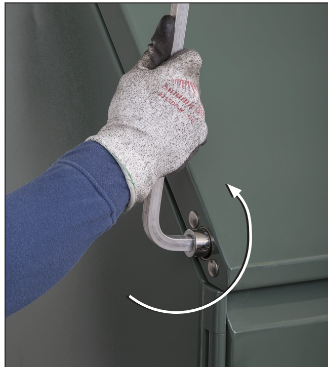
Figure 12. To unlock the hinged roof, turn the pentahead socket wrench 360° counterclockwise .
