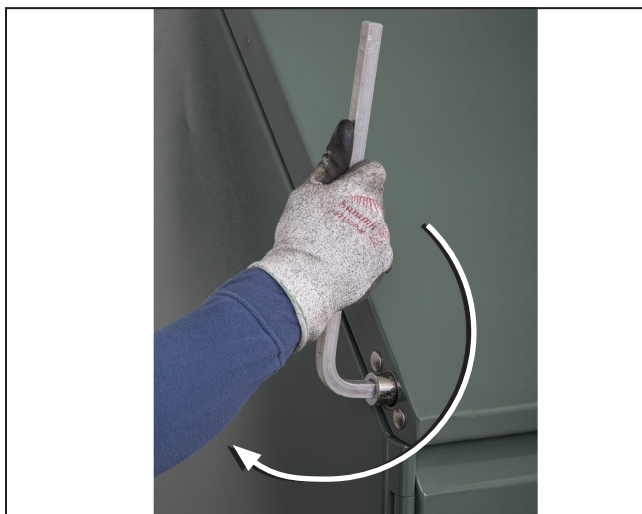
Figure 24. To fully latch the hinged roof, rotate the pentahead socket wrench or tool 360° clockwise.
