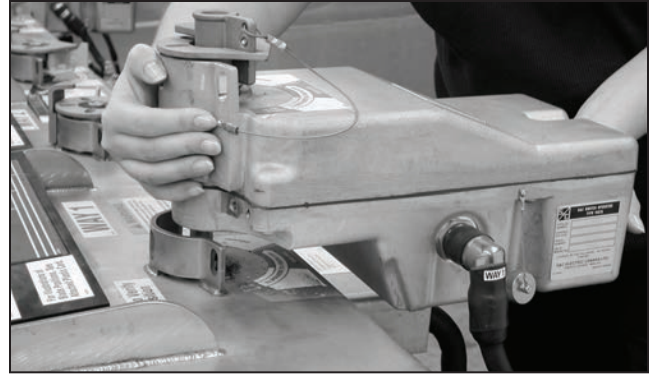
Figure 93. Place the motor operator over the operating shaft on the gear.
