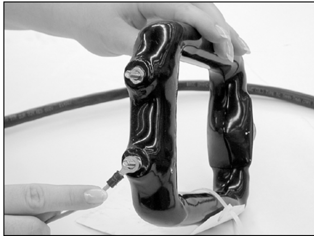
Figure 20. Attach current sensors to required wiring.
