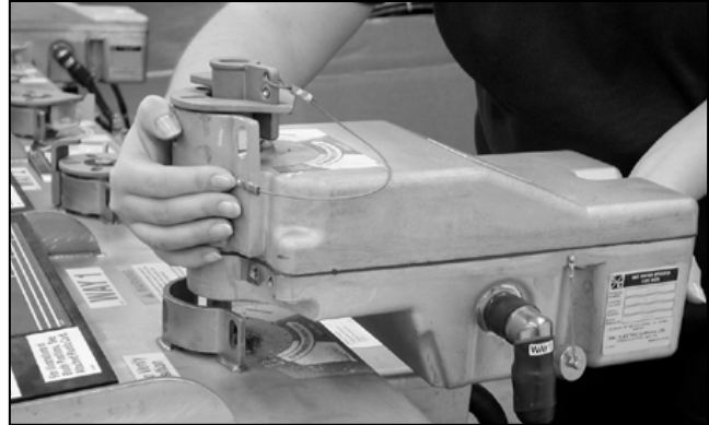
Figure 124. Placing the motor operator over the operating shaft on the gear.
