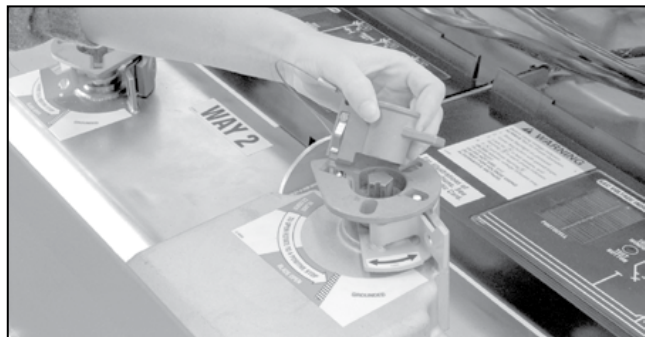
Figure 70. The mechanical blocking key.
