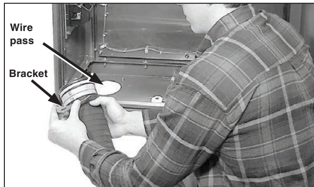
Figure 85. Place the holding brackets in the grooved channel of the conduit.
