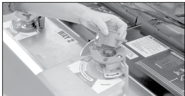
Figure 127. The mechanical blocking key.
