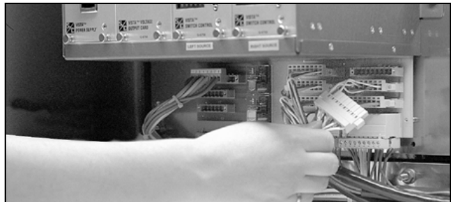
Figure 62. Attaching the connectors to the backplane board.
