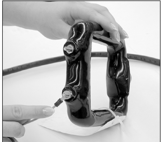
Figure 54. Attach current sensors to required wiring.
