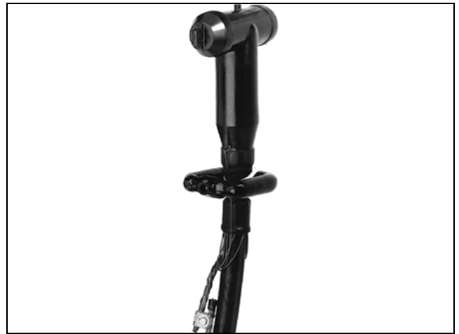
Figure 22. A current sensor placed above the cable’s grounded concentric neutral.
