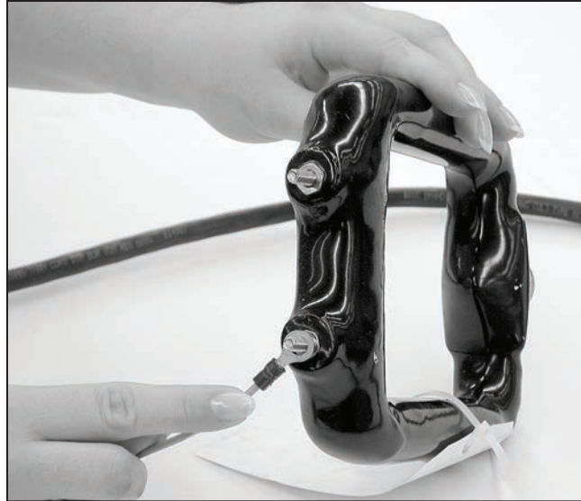
Figure 14. Attach current sensors to required wiring.
