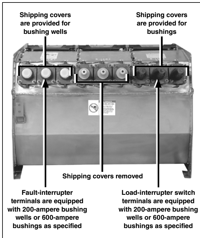
Figure 50. A Vista switchgear tank with shipping covers. (Manual unit shown for illustration purposes.)
