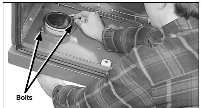
Figure 117. Installing and securing the assembly through the wire pass.
