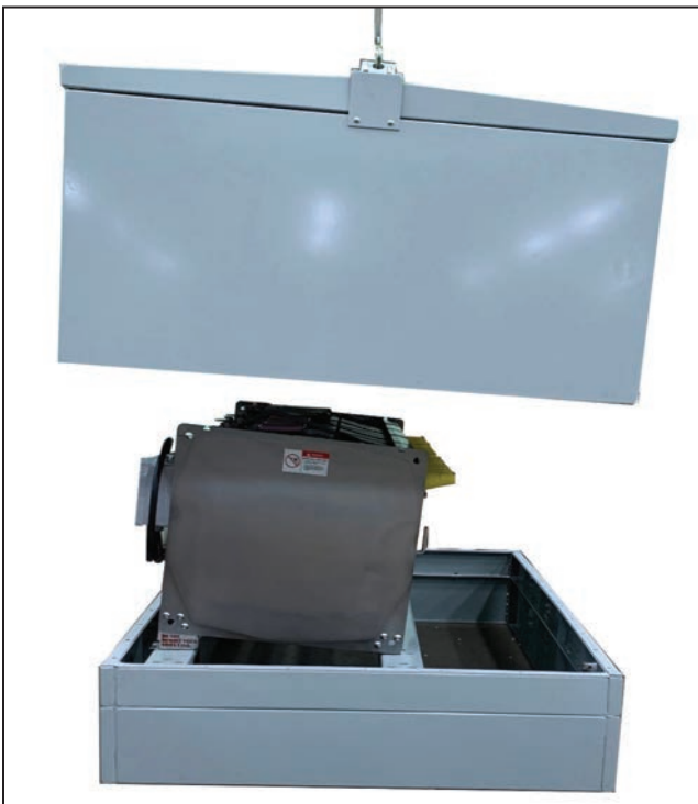
Figure 6. Remove the high voltage enclosure from the base spacer.
