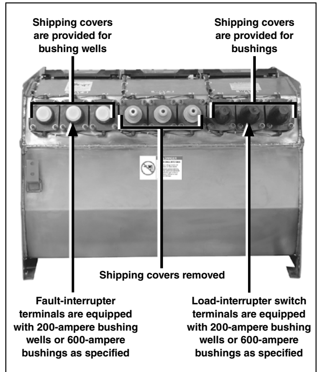
Figure 107. A Vista switchgear tank with shipping covers. (Manual unit shown for illustration purposes.)
