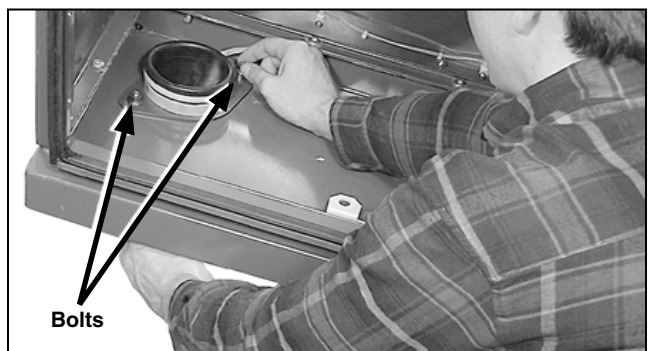
Figure 88. Installing and securing the assembly through the wire pass.
