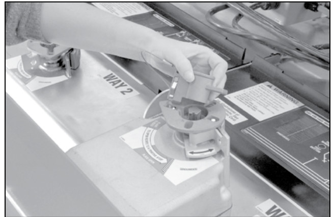
Figure 44. The mechanical blocking key.
