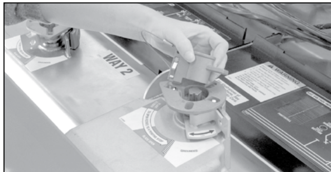
Figure 98. The mechanical blocking key.
