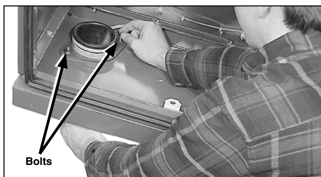
Figure 60. Installing and securing the assembly through the wire pass.
