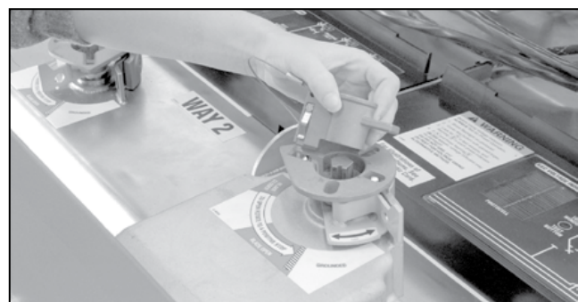
Figure 75. The mechanical blocking key.
