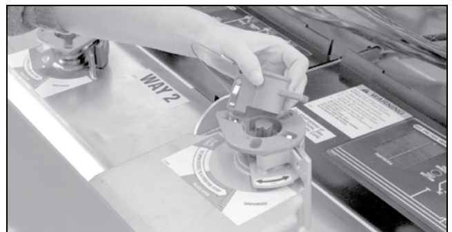
Figure 39. The mechanical blocking key.
