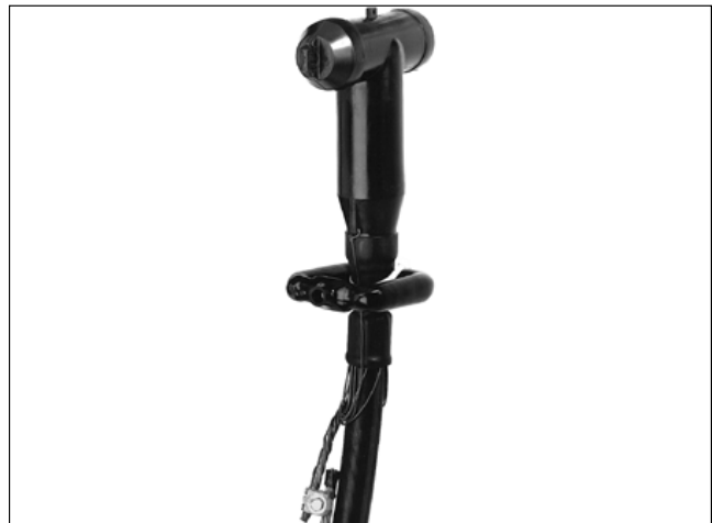
Figure 113. A current sensor placed above the cable’s grounded concentric neutral.●
