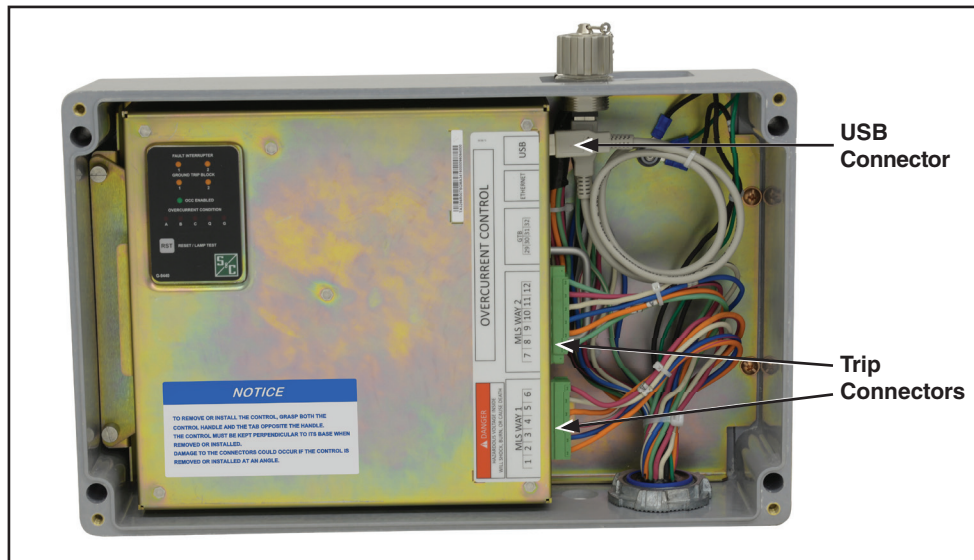
Figure 3. Disconnect the trip connectors and the USB connector.
