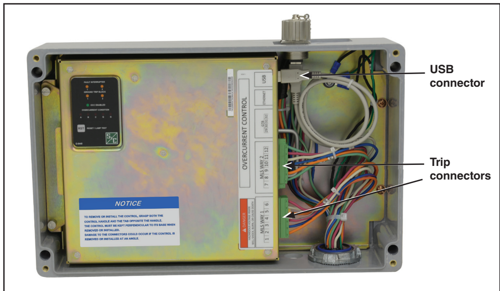
Figure 9. Reconnect the trip connectors and the USB connector to the electronics module and screw them in securely.
