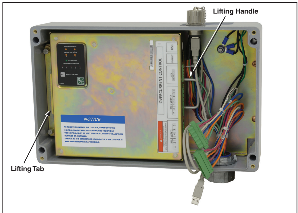
Figure 6. Grasp both the lifting tab and the lifting handle and lift the module up to remove it from the base plate.
