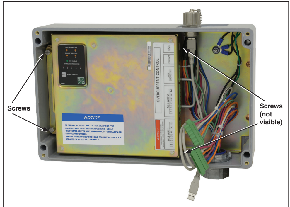
Figure 8. Lower the electronics module onto the base plate and tighten the four captive screws.
