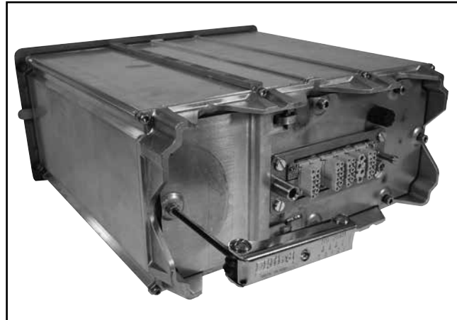
Figure 5. To open the battery compartment cover, loosen the locking screw using a \frac{3}{16} -inch Allen wrench.
