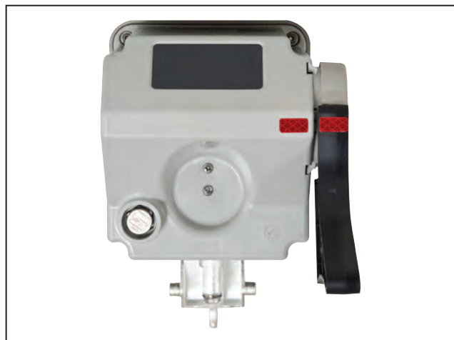
Figure 21. Align the lever with the label on the body.
