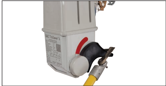
Figure 9. Place the prong above the lever and pull down to enter NR mode.
