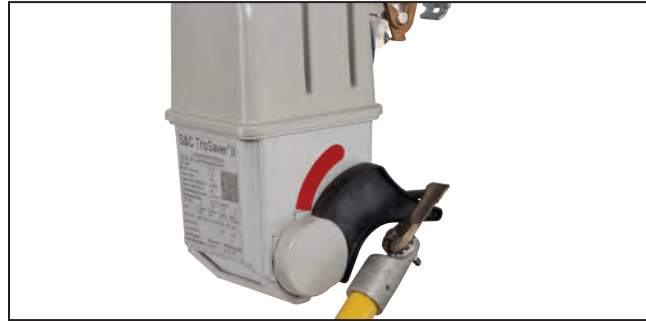
Figure 13. Place the prong above the lever and pull down to enter NR mode.
