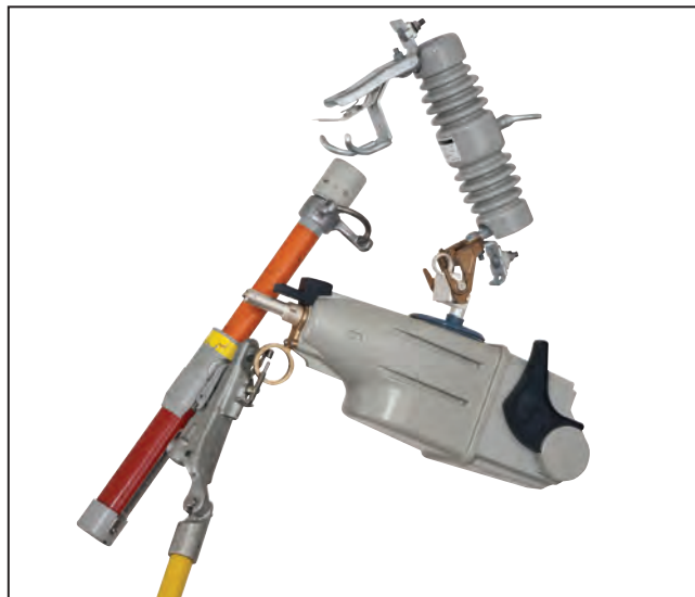
Figure 38. Detaching a Loadbuster tool from a TripSaver II recloser.
