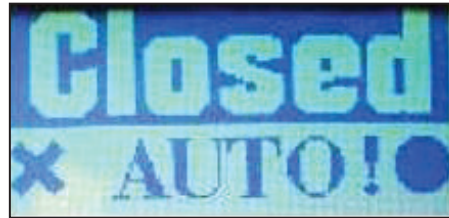
Figure 45. Exclamation point indicator for a battery abnormality.
