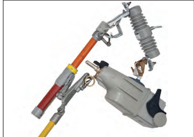
Figure 37. A Loadbuster tool in the Tripped position.
