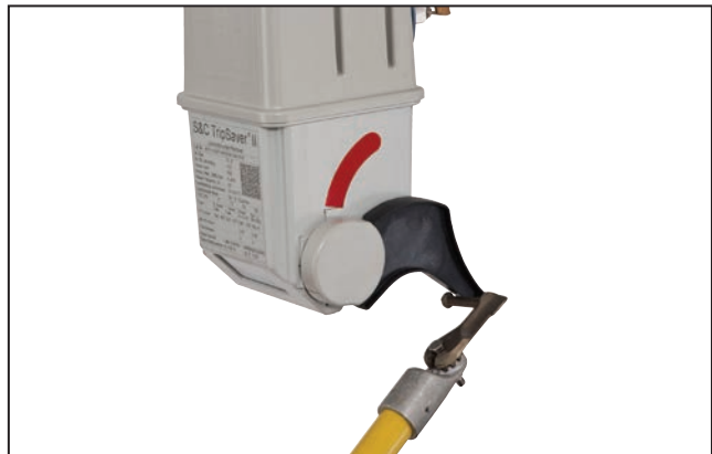
Figure 10. Place the prong under the lever and push up to enter Auto mode.
