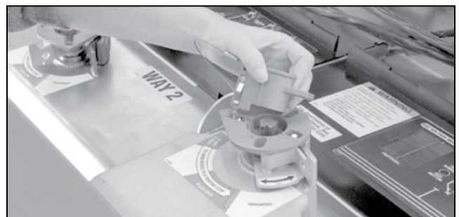
Figure 39. The mechanical blocking key.
