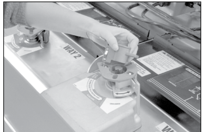
Figure 45. The mechanical blocking key.
