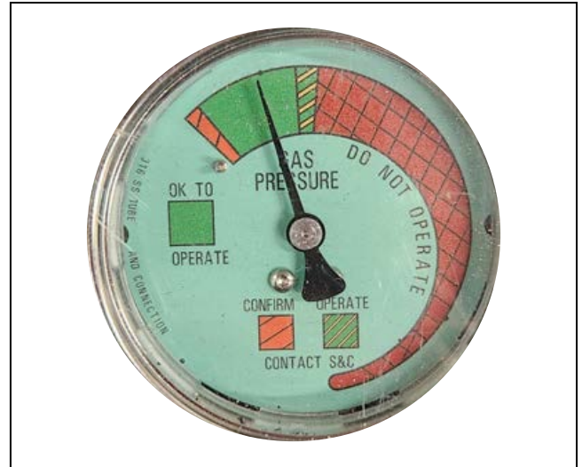
Figure 137. The internal gas-pressure gauge for Vista Green switchgear models (CO 2 mix), “-GRN” catalog numbers.
