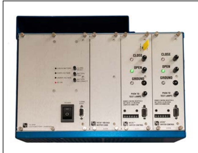
Figure 75. The Open indication on the motor control board matches the motor operator position.
