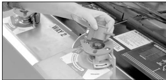
Figure 107. The mechanical blocking key.
