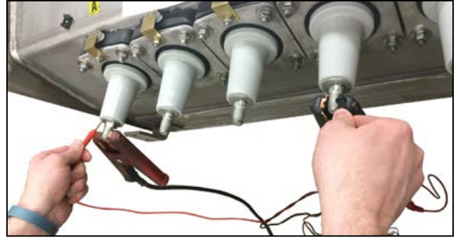
Figure 138. Connecting the resistance measuring device.●
