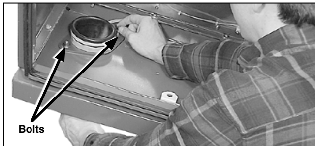
Figure 61. Installing and securing the assembly through the wire pass.
