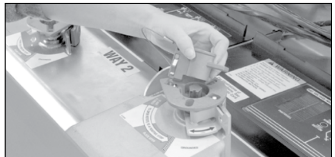
Figure 99. The mechanical blocking key.
