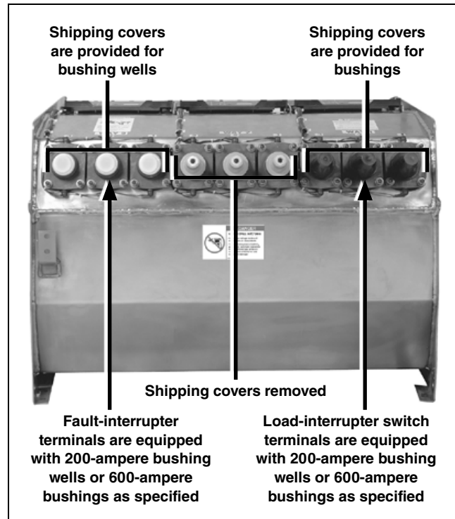
Figure 109. A Vista switchgear tank with shipping covers (manual unit shown for illustration purposes).
