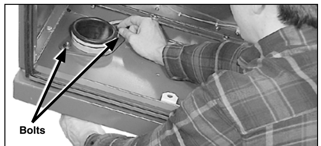
Figure 119. Installing and securing the assembly through the wire pass.
