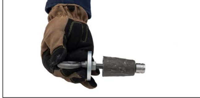
Figure 38. The plug install/removal tool installed onto the plug.
