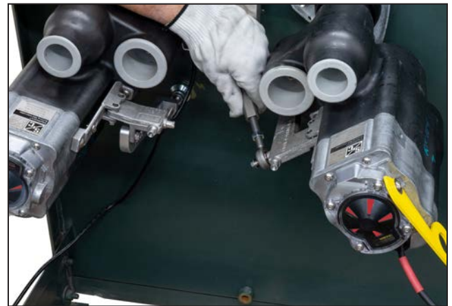
Figure 24. Install a bolt to connect the adjustable link to the swivel foot bracket. Hand-tighten the bolt.
