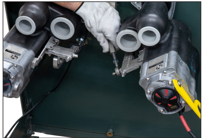
Figure 25. Install a bolt to connect the adjustable link to the swivel foot bracket. Hand-tighten the bolt.
