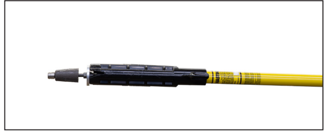
Figure 29. Hold the plug with a shotgun stick or other tool.
