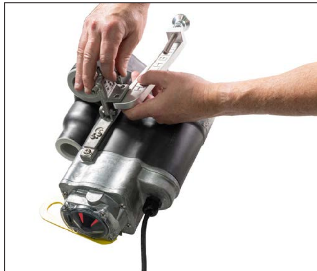
Figure 18. Install the swivel foot on the H1A bushing well interrupter.
