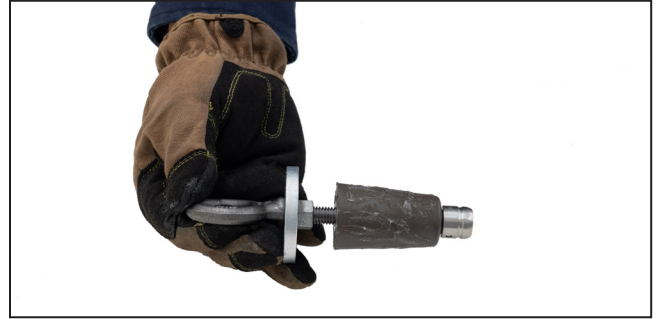
Figure 28. The tool installed onto the plug.
