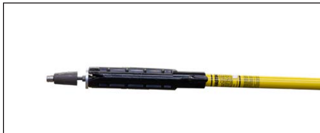
Figure 39. Hold the plug with a shotgun stick or other tool.
