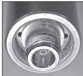
Figure 7. Do not block antenna drain holes.
