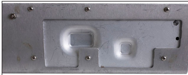
Figure 12. The six new screws that secure the R3 Wi-Fi/GPS module mounting plate.
