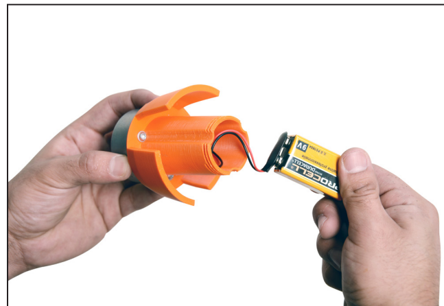
Figure 27. Train the wires inside the body of the module and replace the pull-ring.
