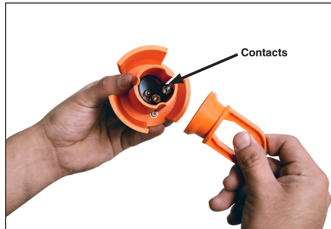
Figure 26. The battery compartment inside the cordless power module.
