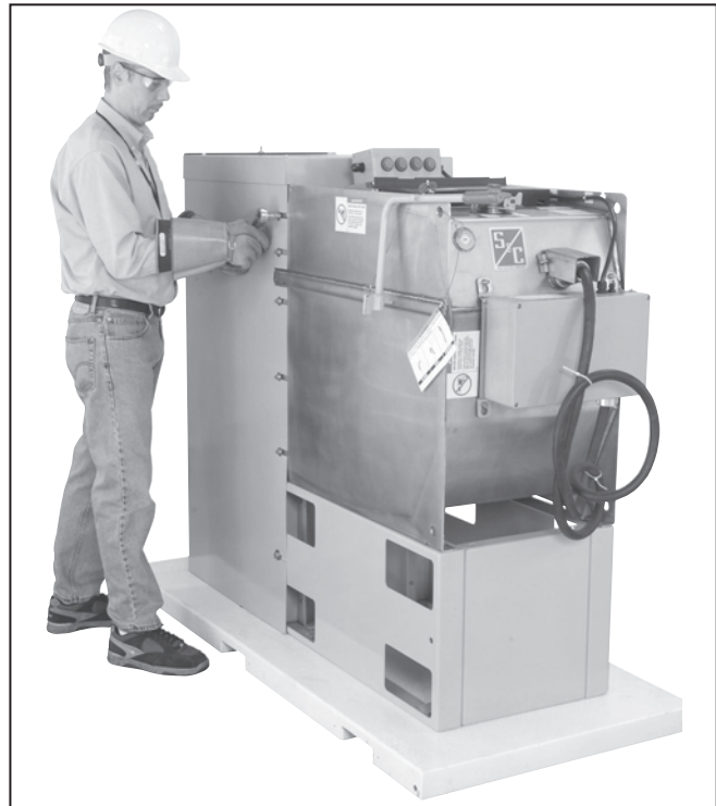
Figure 7. Tighten the six hex nuts that were retained on the studs.
