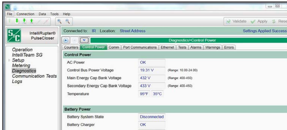
Figure 16. The Diagnostics > Control Power screen.
