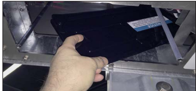
Figure 5. Placing the dust cover in the module bay.
