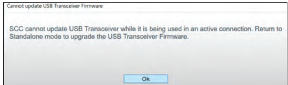
Figure 63. The Cannot update USB Transceiver Firmware dialog box when service center configuration software is in Connected mode.
