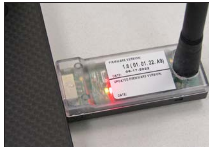
Figure 152. LED indicators on the USB Transceiver.
