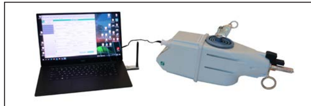
Figure 151. Placement of the TripSaver II recloser in relation to the USB transceiver.
