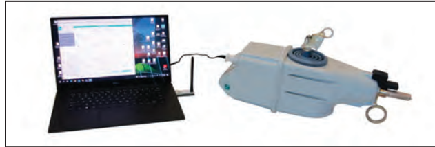
Figure 154. Placement of the TripSaver II recloser in relation to the USB transceiver.
