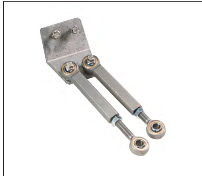
Figure 9. A completed parking stand link bracket assembly.
