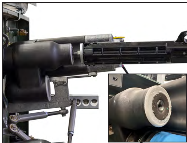
Figure 30. Push into the bushing well interrupter until flush with the bushing well interrupter opening.
