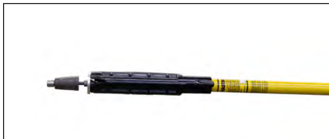
Figure 29. Hold the plug with a shotgun stick or other tool.
