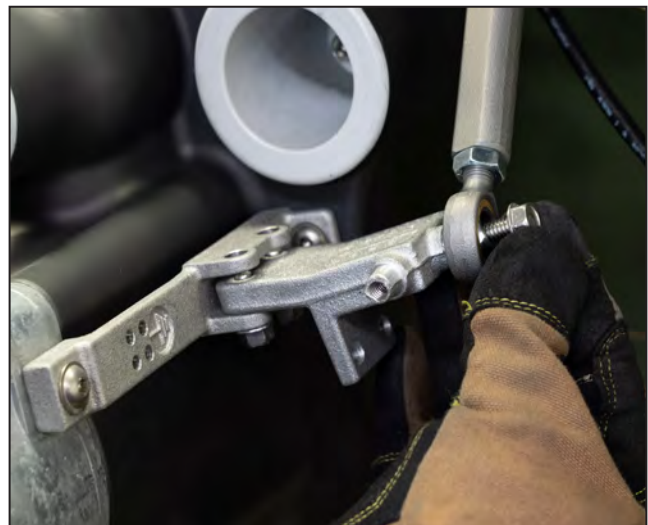
Figure 25. Secure with a flange-head bolt and hand-tighten.
