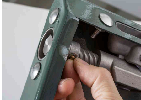
Figure 41. Install a retaining ring on the opposite side of the shear pin.
