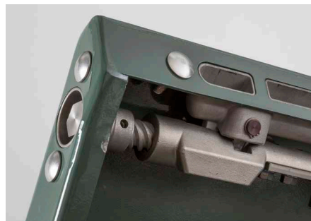
Figure 39. Align hole in plug with the hole in the actuator.
