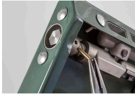
Figure 40. Install the new shear pin.
