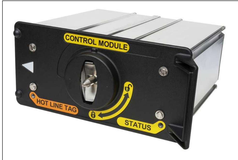
Figure 88. The control module shows the Ready state with a STATUS indicator blink pattern: flashing three times (½ second on, ½ second off) every 30 seconds.
