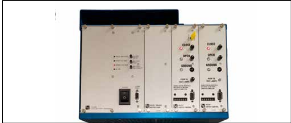
Figure 25. A battery charger with UNDER VOLTAGE indicator illuminated.
