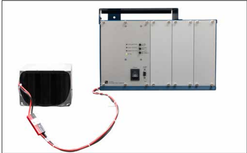
Figure 2. Vista battery charger front panel - AC ON indicator illuminated.
