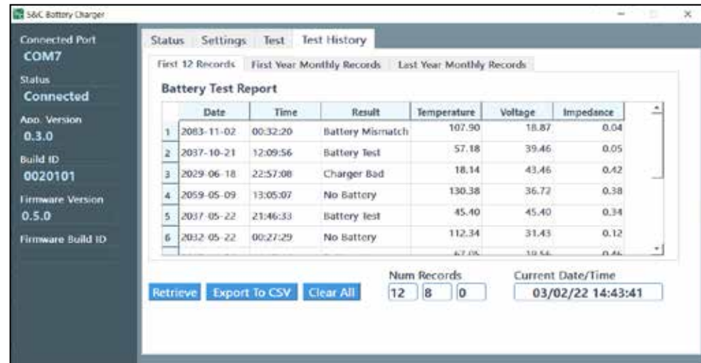
Figure 18. The S&C Battery Charger application Test History tab after retrieving Test History.
