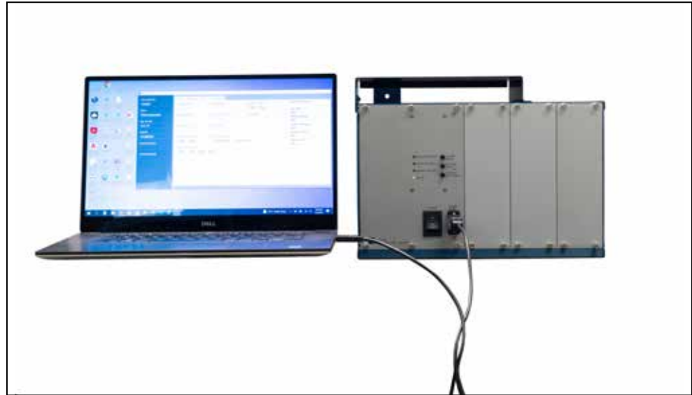
Figure 10. A USB cable connected between a PC and the Vista battery charger.
