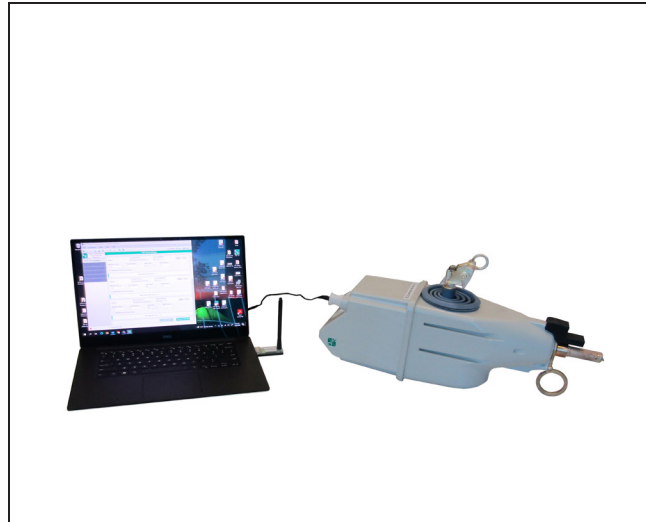
Figure 3. Proper placement of the TripSaver II recloser and USB transceiver for connection.
