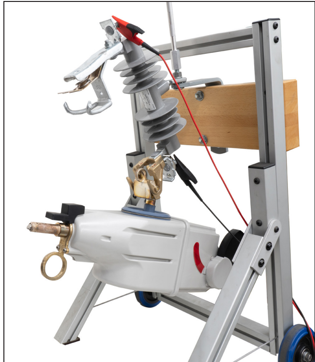
Figure 10. A TripSaver II recloser after dropping out.
