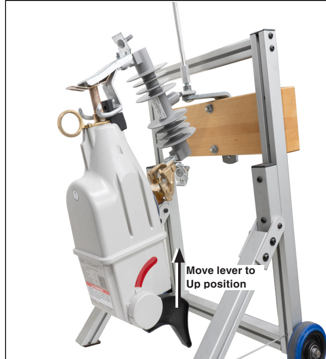
Figure 7. A TripSaver II recloser in the test cutout mounting.
