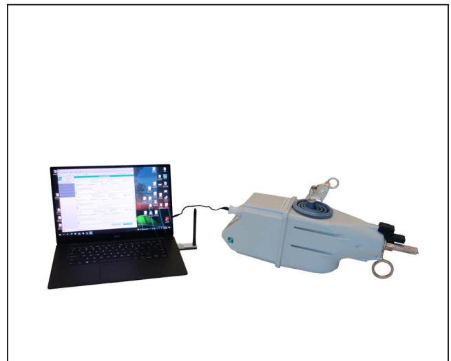
Figure 3. Proper placement of TripSaver II recloser and USB transceiver for connection.
