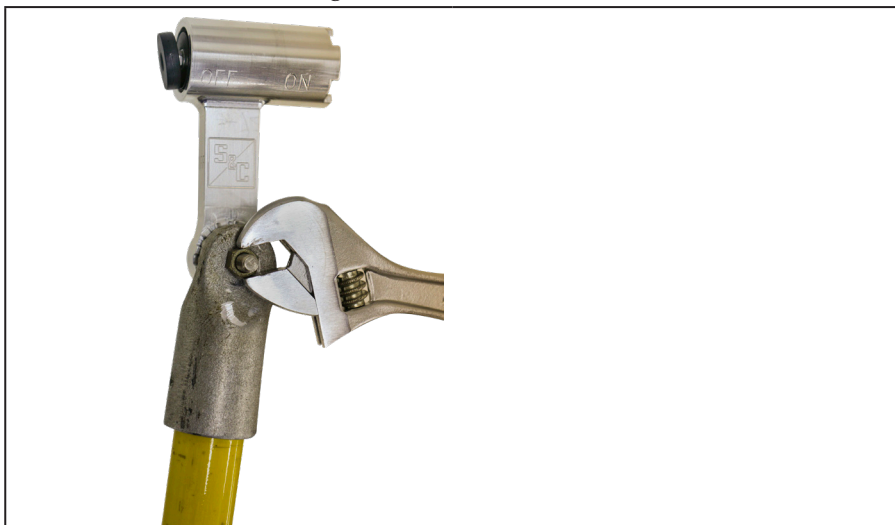
Figure 1. Installing the magnet tool to a hotstick.
