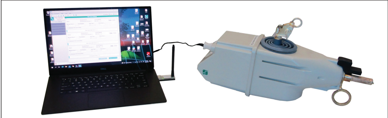
Figure 7. Completed TripSaver II recloser setup.
