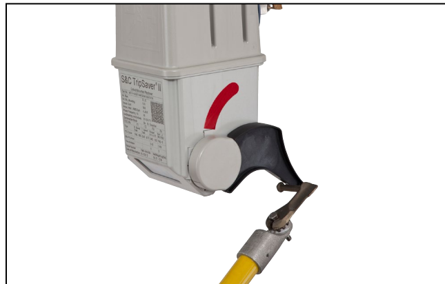
Figure 14. Place the prong under the lever and push up to enter Auto mode.
