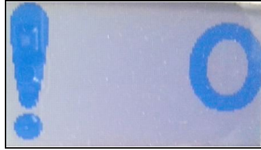
Figure 49. The Service Now screen showing the vacuum interrupter in the Open position.
