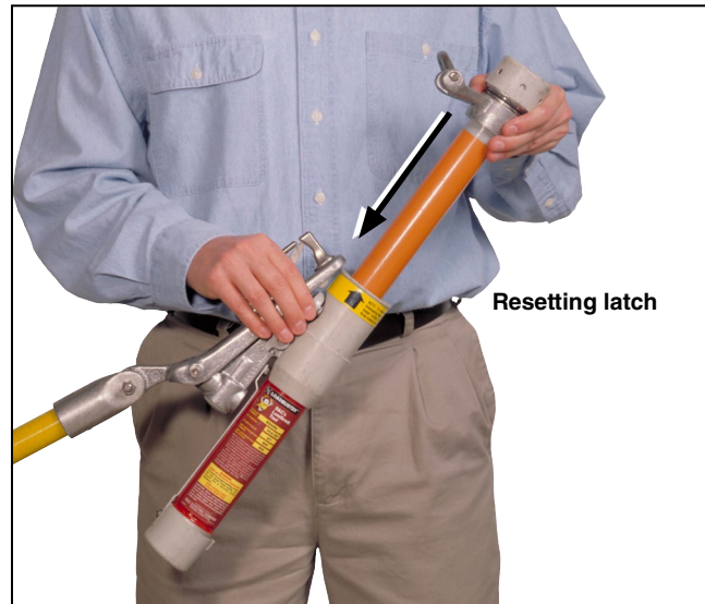
Figure 39. Resetting a Loadbuster tool.
