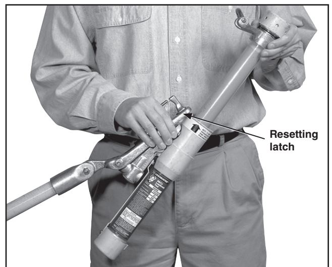
Figure 24. Resetting the Loadbuster Tool.
