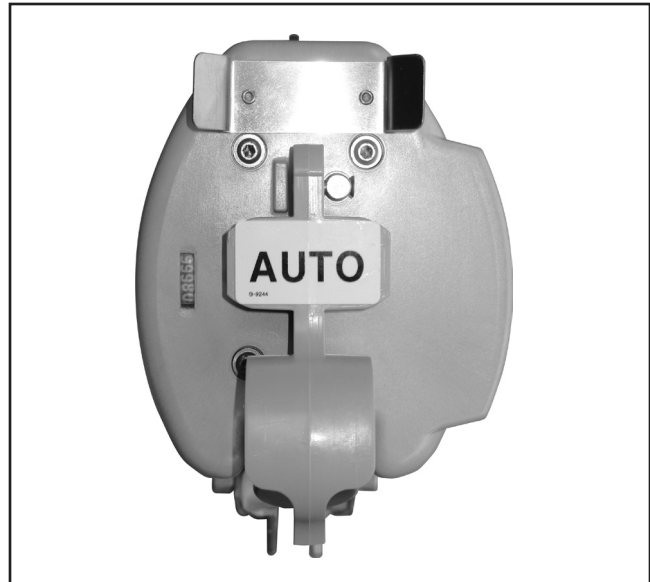
Figure 10. Verifying mode selector handle is in AUTO position.
