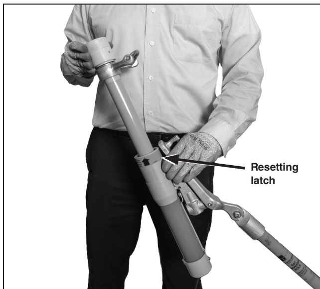
Figure 12. Resetting the Loadbuster tool.
