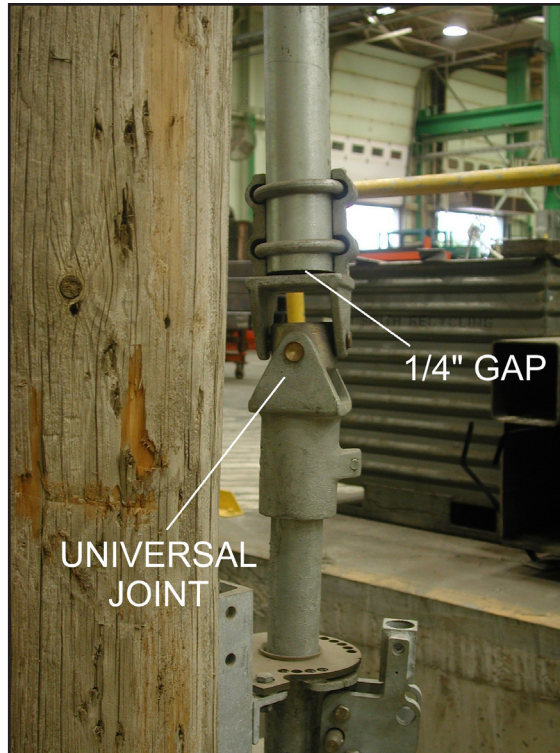
Figure 4. The universal joint showing the 1/4-inch (6-mm) gap for the top pipe.
