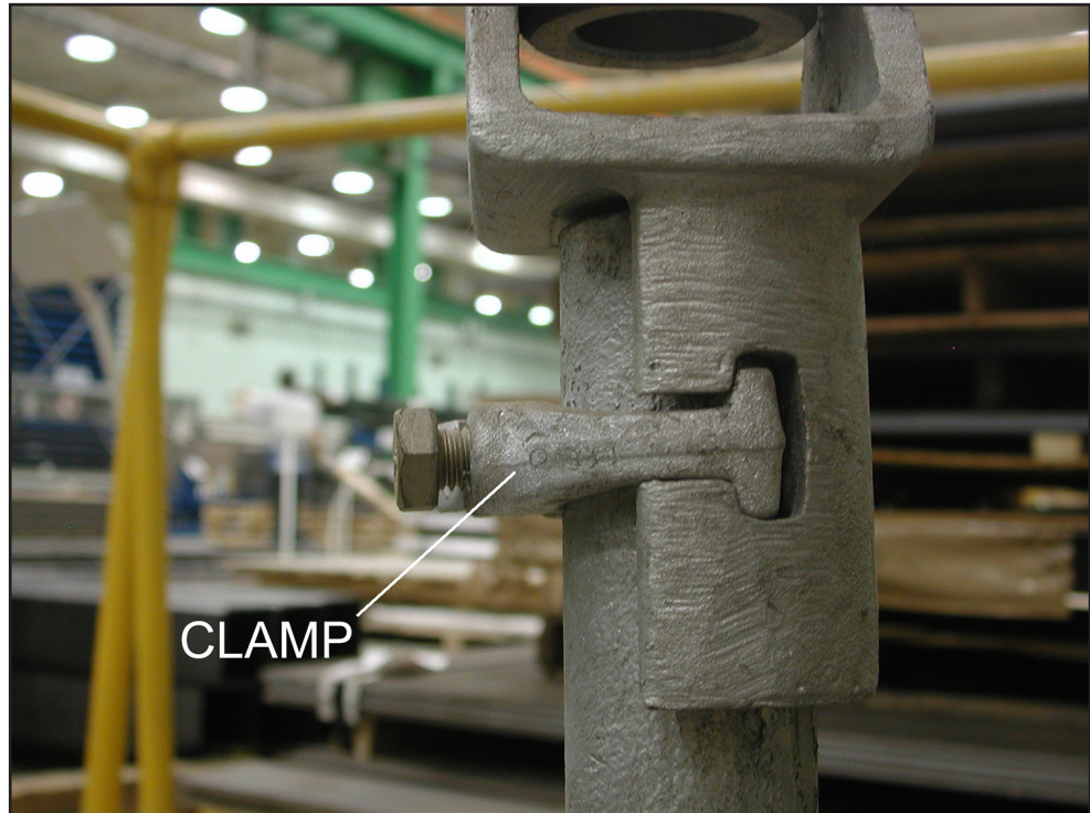
Figure 8. The universal joint clamp at the first section of pipe.
