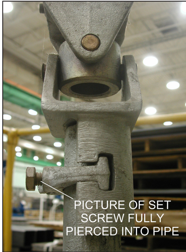
Figure 6. The fully pierced set screw does not need to be flush with the bracket.
