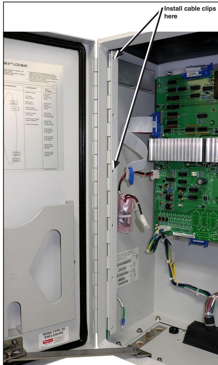
Figure 8. Cable clip locations at the front panel.
