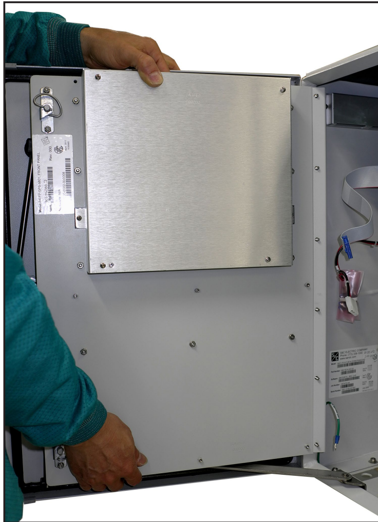
Figure 5. Remove existing front panel.
