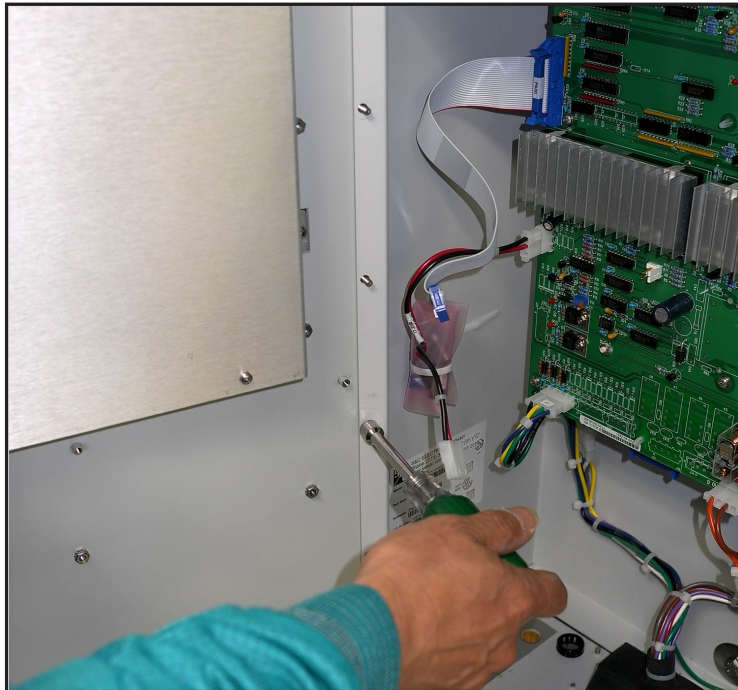
Figure 4. Remove the front panel attachment nuts.
