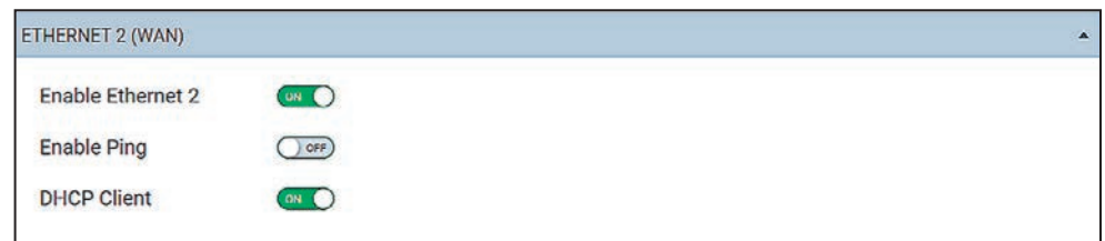
Figure 21. Enable Ethernet 2 set to “ON,” the default.
