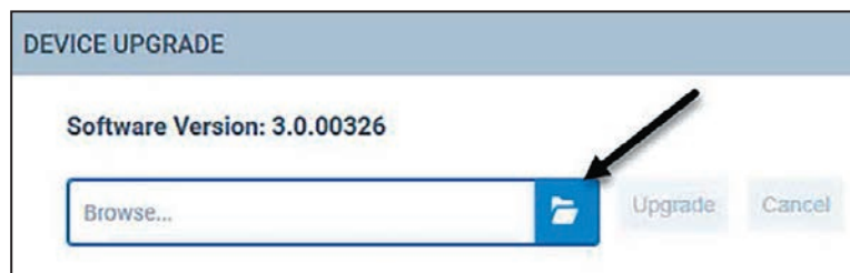
Figure 10. Upload the firmware file to the R3 Communication Module.
