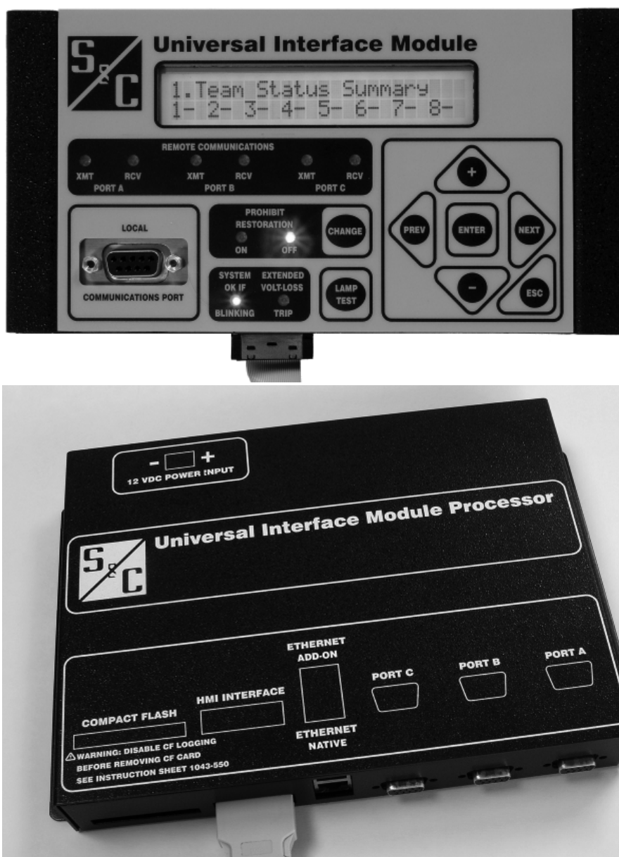
Figure 1. Remote faceplate and main chassis of the Panel-Mounted Universal Interface Module.
