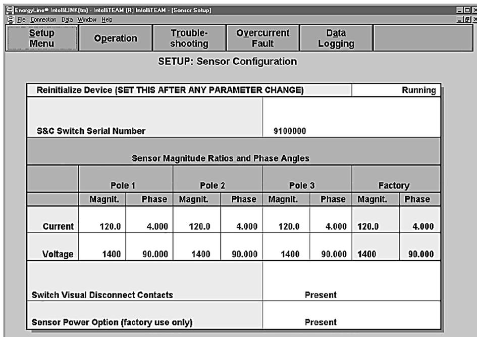
Figure 6. The *Setup>Sensor Configuration* screen for a 5801 control.
