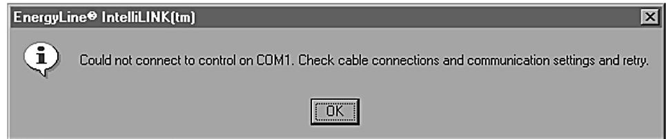
Figure 2. The dialog box displayed when IntelliLink software does not establish communication.
