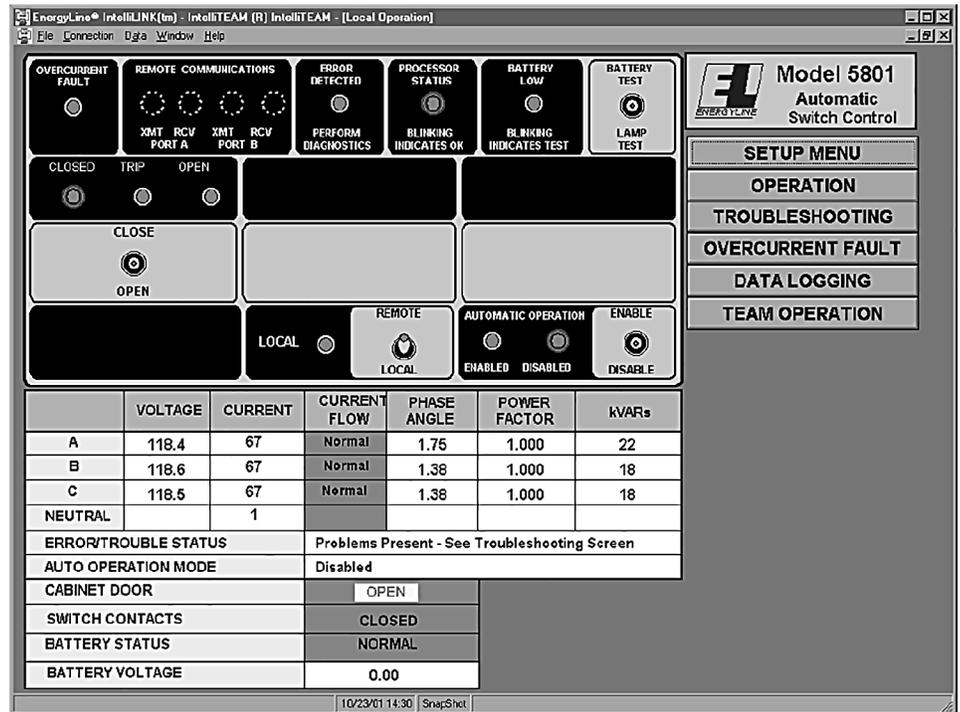
Figure 1. The *Operation* screen for a 5801 Switch Control.
