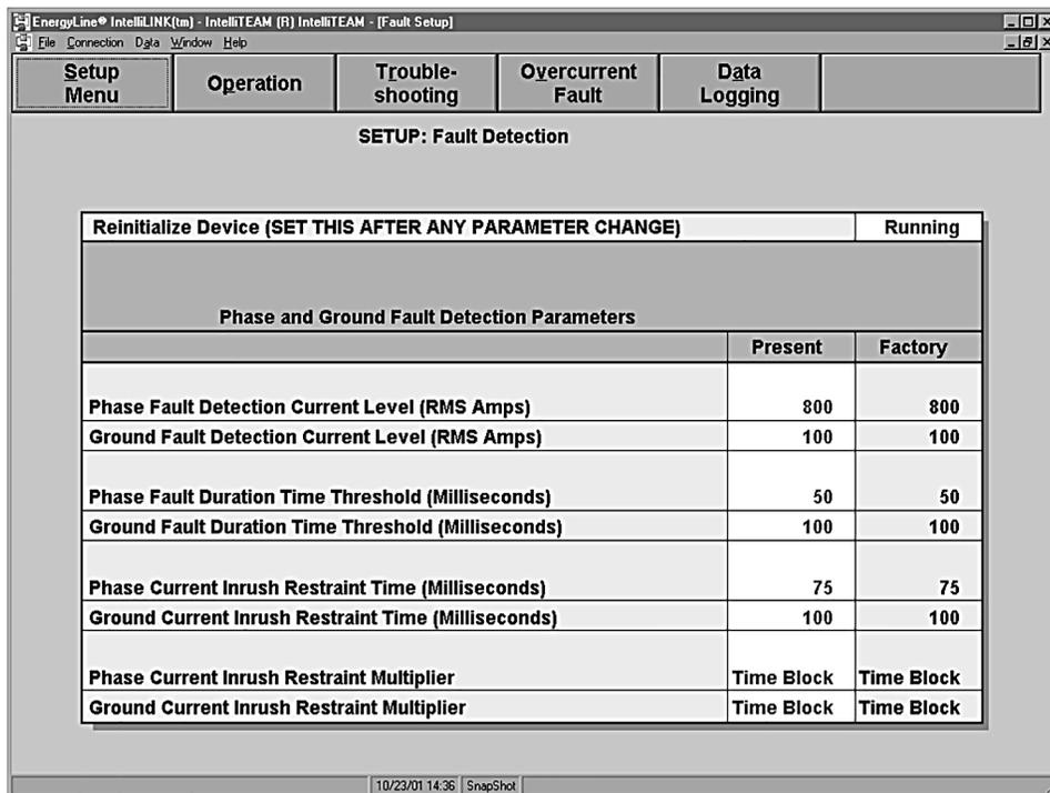
Figure 9. The *Setup>Fault Detection* screen.
