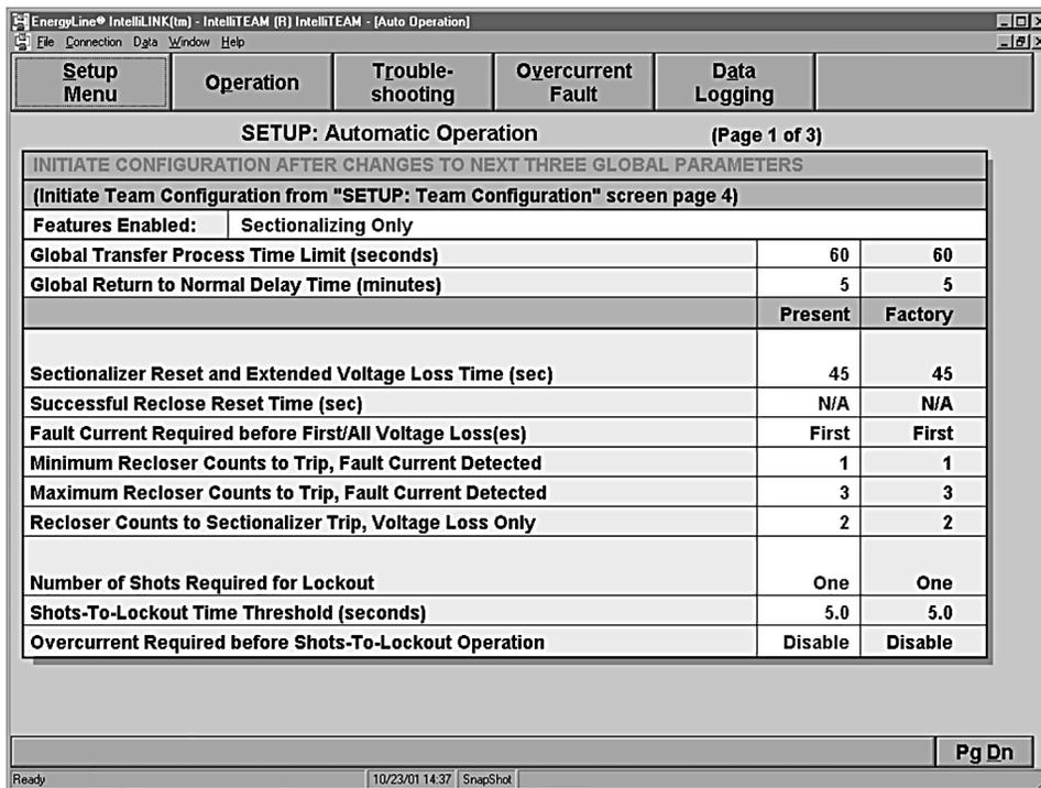
Figure 13. Page 1 of the *Setup>Automatic Operation* screen for a 5801 control.
