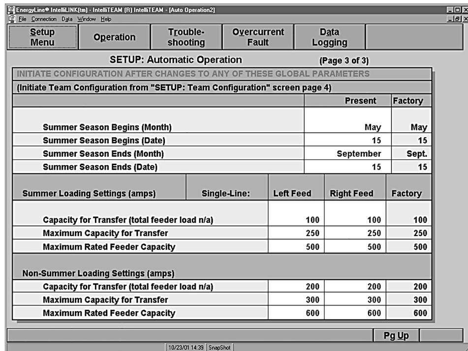
Figure 15. Page 3 of the *Setup>Automatic Operation* screen for a 5801 control.
