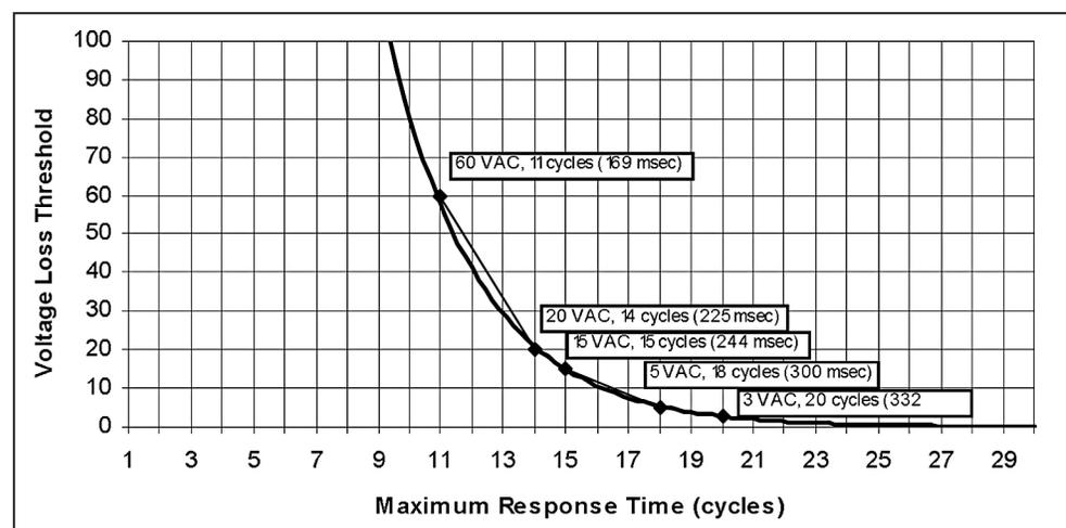
Figure 8. Voltage-Loss Threshold and Maximum Response Time.
