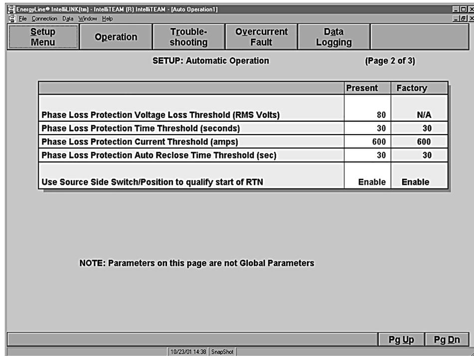
**Figure 14.** Page 2 of the *Setup>Automatic Operation* screen for a 5801 control.
