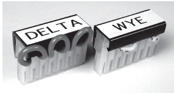
Figure 2. The delta jumper and wye jumper.
