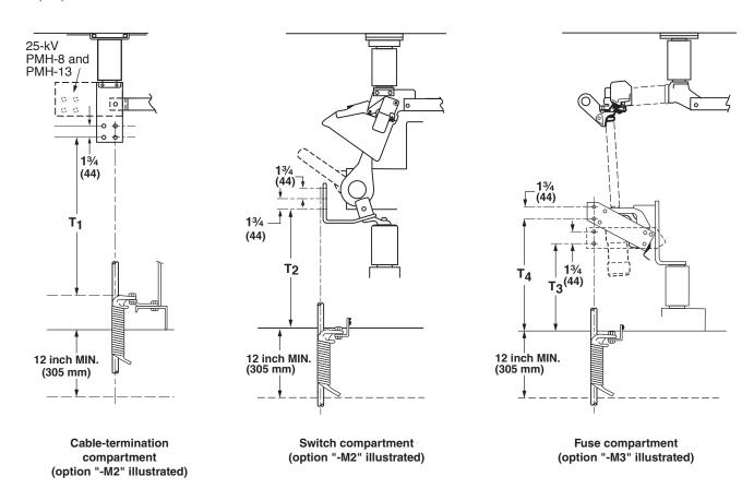
★ These devices extend below the base of the unit. Provide a cable pit, or specify a base spacer that provides a 12-inch (305-mm) or greater increase in elevation of ungrounded parts above the mounting pad.
