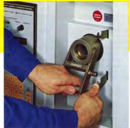
Figure 11. Decoupler handle moves upward to decouple . . . downward to couple.
